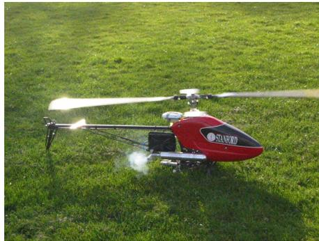
Figure 4: An autonomous XCell Tempest helicopter from Stanford University. The simulator used in the Helicopter Hovering domain is based on real data captured from such helicopters.
